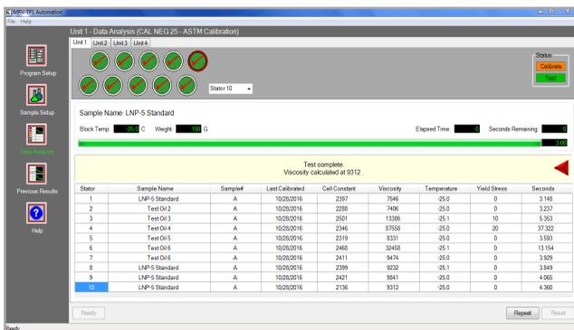
The King MRV Automation Software Package calculates yield stress, viscosity, and Rotor/Stator Cell Constants. It offers simple user prompts to facilitate the testing process and comes installed on the laptop computer.
